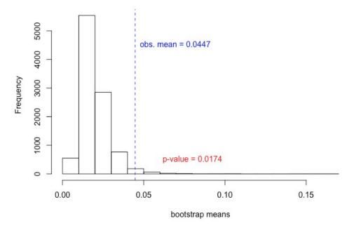
Figure 2. Histogram of 10,000 bootstrapped mean concentrations for a true mean concentration set at 0.02. The dashed blue line shows the value of the observed mean of 0.0447.
