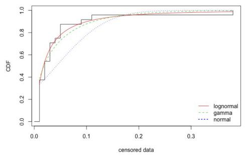
Figure 1. Three distributions (smooth curves) fit to the atrazine data (step function)
